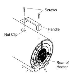
Figure 5 - Attaching Handle
